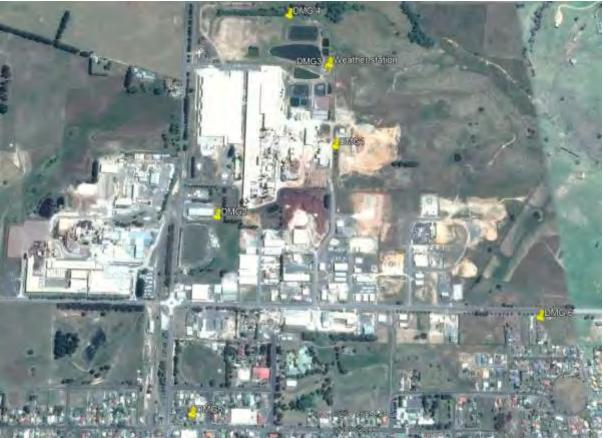
Figure 5 Depositional Dust Gauge Locations
